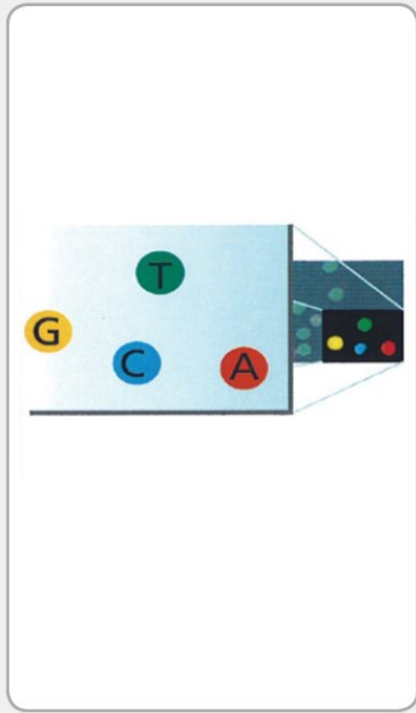
After laser excitation, capture the image of emitted fluorescence from each cluster on the flow cell. Record the identity of the first base for each cluster.
